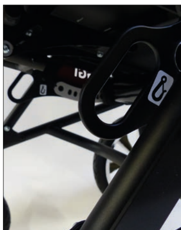
Attachment points, front according to ISO 7176-19
