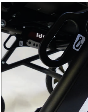
Attachment points, front according to ISO 7176-19
