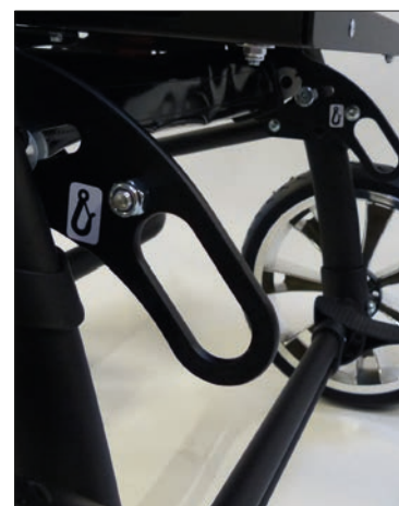
Attachment points, rear according to ISO 7176-19
