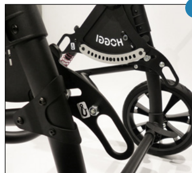
Tie down kit according to ISO 7176-19
