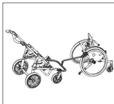
Connecting parts for coupling a BINGO Evolution mobility base and a HOGGI wheelchair
