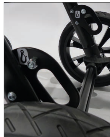
Attachment points, rear according to ISO 7176-19
