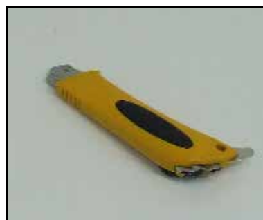
Carpet knife with sickle and standard blade
