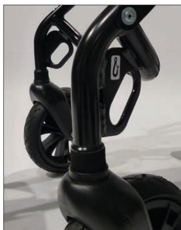
Attachment points, front according to ISO 7176-19
