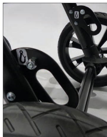
Attachment points, rear according to ISO 7176-19
