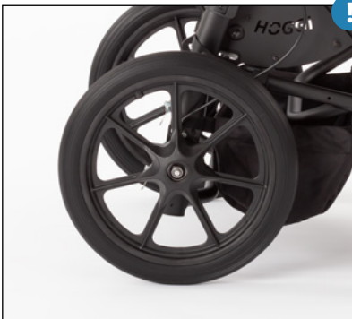
Drum brake wheels with tyres on black 5-spoke rims, with locking function
