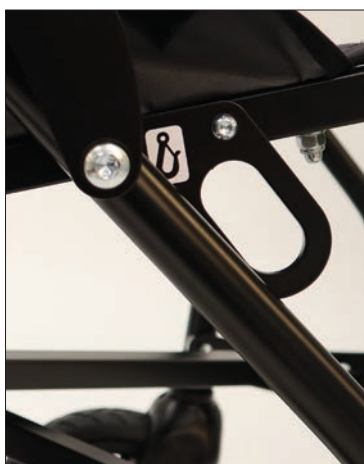
Attachment points, front according to ISO 7176-19
