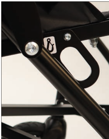
Attachment points, front according to ISO 7176-19
