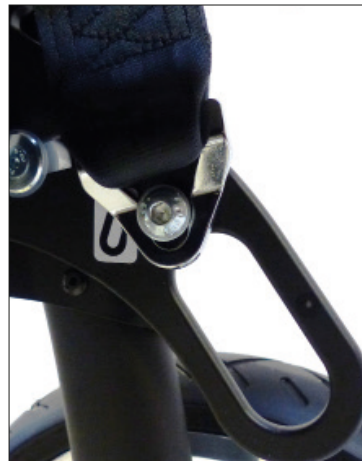
Attachment points, rear according to ISO 7176-19 for lap belt
