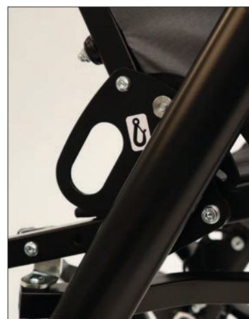
Attachment points, rear according to ISO 7176-19
