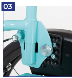
03 Back base, foldable and angle adjustable
