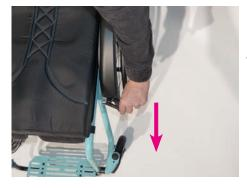
• To open the *HOGGI* light brake, push the brake lever forward as shown.
