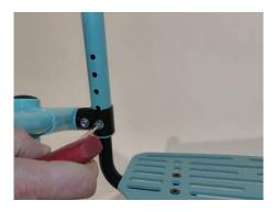
• Loosen and remove the screw connections on both sides.
