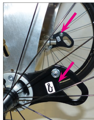
Attachment points, rear according to ISO 7176-19
