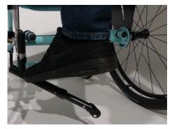
• Turn the anti-tip with the foot to the inside until the inactive position is reached.
