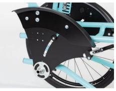
**Seat height**, **seat depth** and **seat angle** will be adjusted on the base plates.
