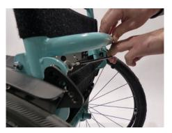
• Pull the release rope with one hand as shown and move the back construction backwards with the other hand.
