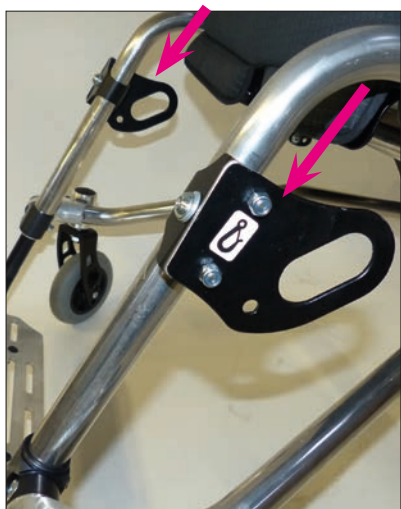
Attachment points, front according to ISO 7176-19
