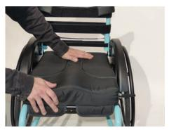
• Press the cushion on the seat panel and the Velcro strips as shown.
