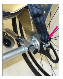
Attachment points, rear according to ISO 7176-19 for lap belt
