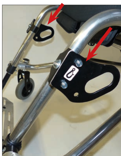
Attachment points, front according to ISO 7176-19
