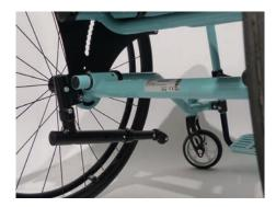
The illustration shows an anti-tip in the "inactive position".
