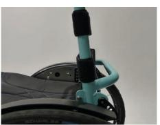
• Engage both bolts audibly in the desired back angle position.
