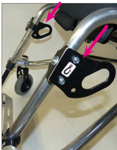
Attachment points, front according to ISO 7176-19
