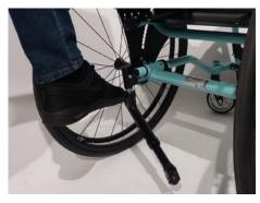
• Turn the anti-tip with the foot to the inside into the active position.
