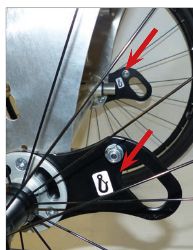
Attachment points, rear according to ISO 7176-19
