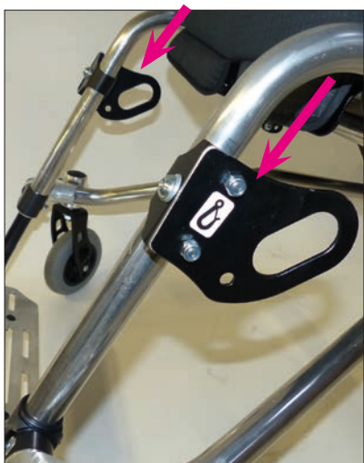
Attachment points, front according to ISO 7176-19
