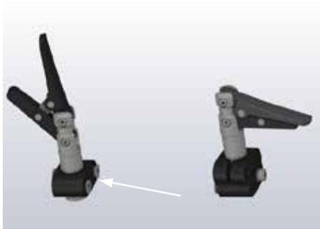
Check of the screw connections:
