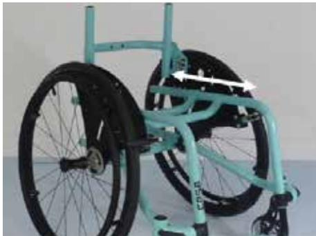
The frame can now be adjusted to the appropriate depth
