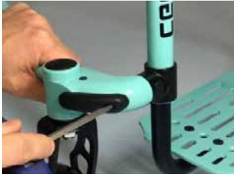
Check the screw connection between the beams and the seat frame.
