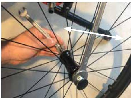
Adjustment of the quick-release axle:
