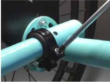
Loosen the screw connection on the right and left at the clamps of the axle tube.
