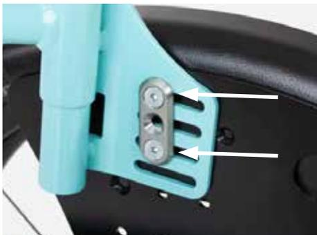
If CESA is not equipped with the backrest base „angle-adjustable and foldable“, the backrest angle is adjusted by loosening the marked screw connection.
