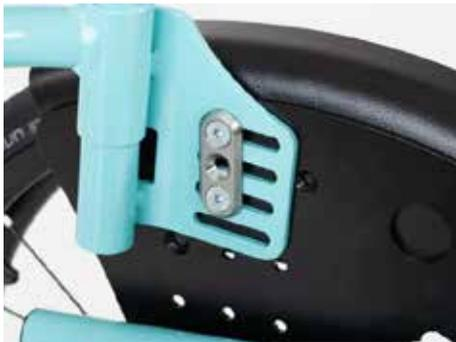
The elongated holes in the back base give an adjustment range of 3 cm. This results in a total adjustment range of 5 cm + 3 cm = 8 cm.
