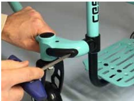
Finally, tighten the side screw connection again.
