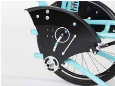
Then, by loosening the screw connection to the base plate, move the seat frame up and down within the slotted hole and thus adjust or adapt the seat angle/rear seat height. Then tighten the screw connection again. 0° - 12° adjustment range
