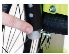
Make sure, that both spring buttons clicked into position below the locating brackets.
