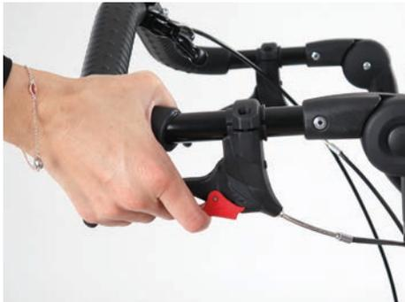
When the brake lever is squeezed again, the rocking catch is unlocked and the drum brake can be released.
