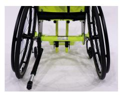
The length of the tubes can be adjusted in three positions.
