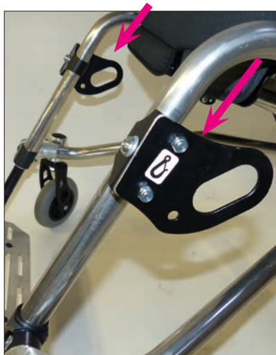
Attachment points, front according to ISO 7176-19
