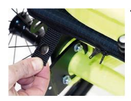
• Fasten the flap of the seat cushion to the back edge of the seat surface and fix it with the press button.
