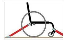
The attachment points of the pushchair restraint systems are marked with the international hook symbol.
