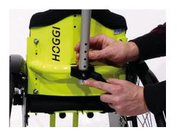
• Press in the spring button and slide the one hand push-handle until it clicks into position.
