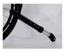
Press the snap button and choose the desired length position. The length of the anti-tipper tubes can be adjusted in the anti-tipper bracket in three positions 2.5 cm apart.
