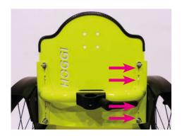
The backrest height can also be adjusted infinitely variable after loosing the marked screw connections (on both sides) within the slotted holes.
