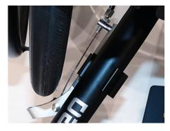
When the wheel lock is released the brake shoe should be 12-15 mm from the wheel.
