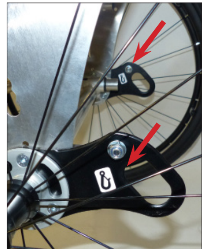
Attachment points, rear according to ISO 7176-19
