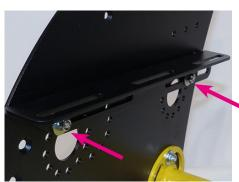
Loosen and remove the marked screw connections on both sides
