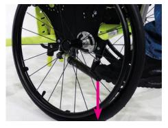
• Turn the anti-tip with the foot to the inside until the inactive position is reached.
