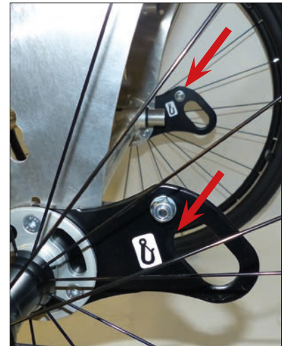
Attachment points, rear according to ISO 7176-19
