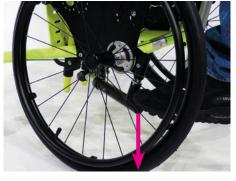
The active position is reached if the anti-tip is snapped audibly.
