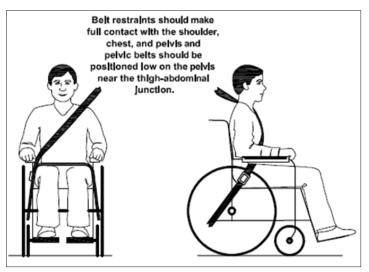
3) The angle between lap belt and horizontal has to be 30°-75°. An angle close to 75° is preferable.
