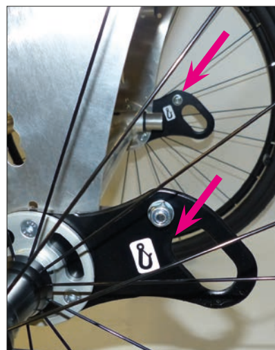
Attachment points, rear according to ISO 7176-19
