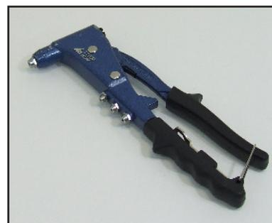
Riveting pliers for rivets up to
