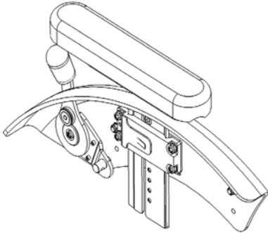
Fender with integrated brake system and armrests
