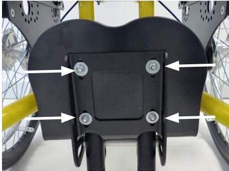
After loosening the four marked screw connections on the footrest bracket, the footrest can be adjusted in depth.
