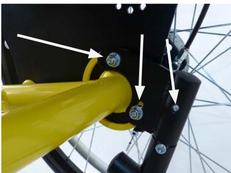
Check of the screw connections:
