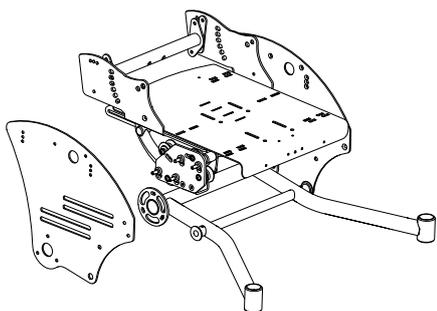
4. To change the seat height, remove the seat unit from the slots and insert it in the desired position.
