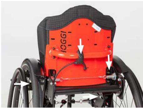
Check of the screw connections:
