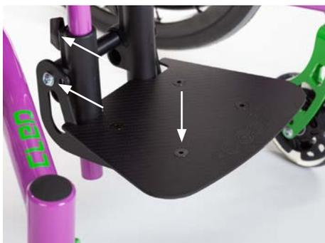
Check of the screw connections:
