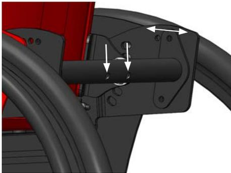
The central push handle holder is attached using the holes in the cross strut.
