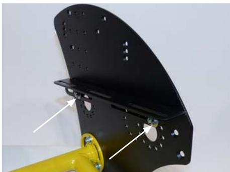
Check of the screw connections:
