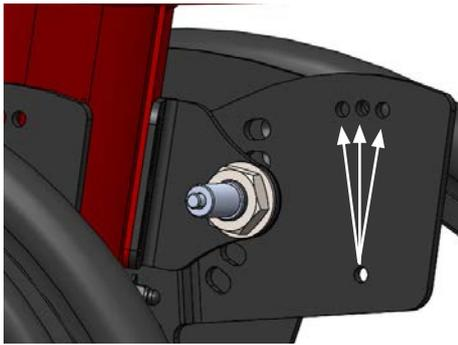
The central push handle can generally be aligned in 3 different positions, depending on whether it is to be aligned further forward or backward.
