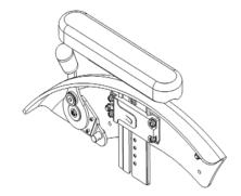
Fender with integrated brake system and armrests
