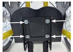
After loosening the four marked screw connections on the footrest bracket, the footrest can be adjusted in depth.
