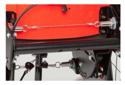
The backrest angle is adjusted by means of a locking bolt on the back.
