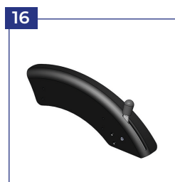
Fender with integrated brake system
