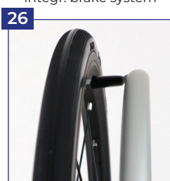
Push rims aluminium anodised, standard
