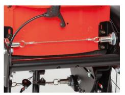
The back angle is adjusted via a locking bolt on the rear.
