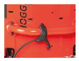
The unit is operated via a release lever on the crossbar of the back support.
