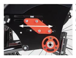
With the **CLEO Ti**, the active degree is achieved by moving the seat unit relative to the base plates in the respective slotted holes.
