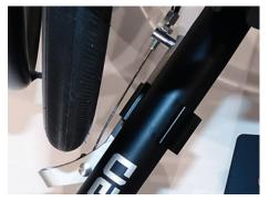
• To open the brake, pull the brake lever upward with your fingers or the ball of your hand.
