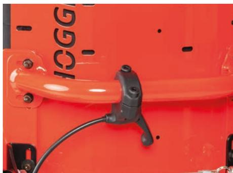
The unit is operated via a release lever on the crossbar of the back support.
