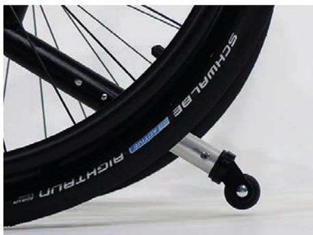
The anti-tip should be adjusted that it is 2-3 cm above the ground.
