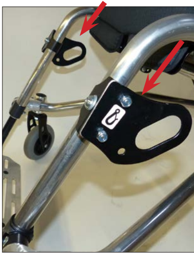
Attachment points, front according to ISO 7176-19
