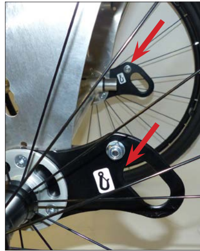
Attachment points, rear according to ISO 7176-19
