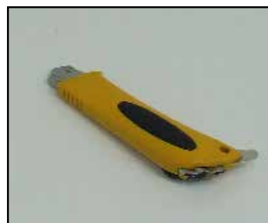
Carpet knife with sickle and standard blade
