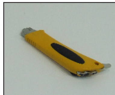
Carpet knife with sickle and standard blade
