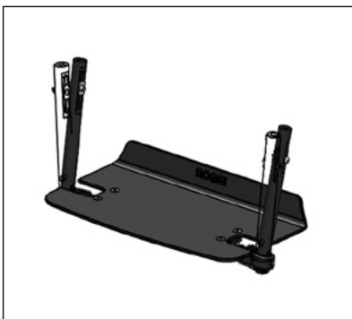
Alu-footboard one piece with heel stop, angle-adjustable, fold-up, LLL 26 - 37 cm
