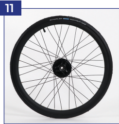
11 Standard rear wheel with drum brake
