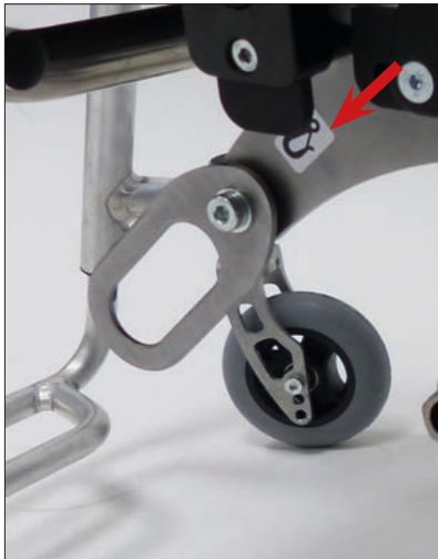
Attachment points, front according to ISO 7176-19
