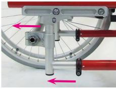
The active degree describes the relation of the backrest position to the rear wheels. The more the backrest is positioned to the rear of the axle, the more active the **SWINGBO-2** can be driven. (e.g. lifting of the front wheels). That means contrary a safer driving position if the adjustment is set above or in front of the rear axle. The active degree is adjustable in 6 steps (0-5) by sliding the axle unit
