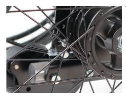
The brake force can be adjusted by the adjustment screw.
