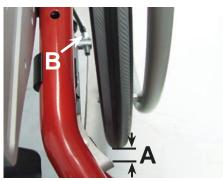
When the wheel lock is released the brake shoe should be 12-15 mm
