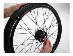
Whilst pressing the release knob, position the quick-release axle into the rear wheel bearing.
