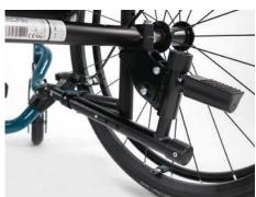
If your **SWINGBO-2** is supplied with an anti tip it is directed to the front. That is the non-active position.
