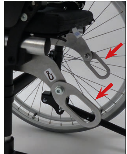
Attachment points, rear according to ISO 7176-19
