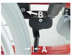
• To release the wheel lock pull the brake lever upwards.
