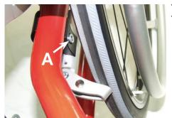
The brake shoe presses on the tires and grips it tightly. The brake shoe is, therefore, at a 90° angle to its holder.
