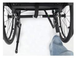
• To adjust the "active position" push the anti-tip with your foot to the bottom.
