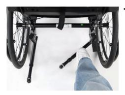
• Turn the anti-tip to the left as shown in illustration 11. (if the anti-tip is mounted on the left side turn it to the right side).
