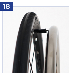
Push rims stainless steel, standard
