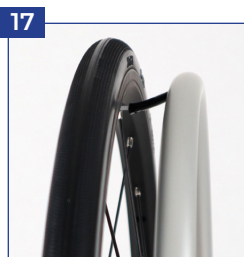
Push rims aluminium anodised, high
