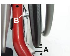
When the wheel lock is released the brake shoe should be 12-15 mm from the wheel (**A**).
