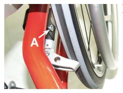
The brake shoe presses on the tires and grips it tightly. The brake shoe is, therefore, at a 90° angle to its holder.
