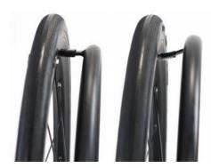
Hand rims can be supplied with a standard diameter (left) or with a larger diameter (right). These are called respectively hand rims "standard" or hand rims "high".
