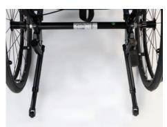
The **SWINGBO 2 XL** wheelchair can be supplied with one or with two anti-tippers.
