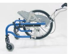
By using the push-bar or push-handles, the seat unit can be adjusted to any angle between -7° and +45°. Set the required seat angle and allow the bolt to lock in the required position.
