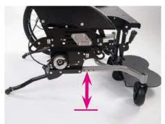
The seat height depends on the chosen rear wheels and front castors as well as on the height of the rear axle and the position of the front castors in the front castor forks.
