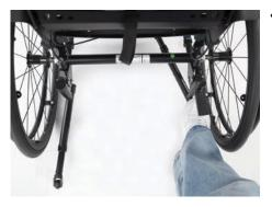
To adjust the "active position" push the anti-tip with your foot to the bottom.
