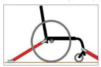
4) The buggy has to be fixed with a restraint system referred to ISO 10542 or SAE J2249 with fixed belts in the front and adjustable belts in the back.
