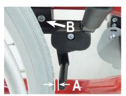
• To release the wheel lock pull the brake lever upwards (25).
