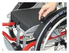
To release the wheel lock pull the brake lever upwards as shown.
