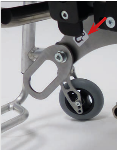
Attachment points, front according to ISO 7176-19
