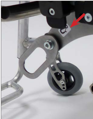
Attachment points, front according to ISO 7176-19
