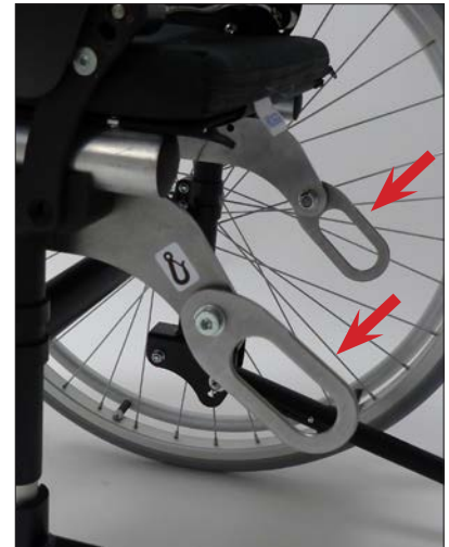
Attachment points, rear according to ISO 7176-19
