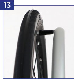
13 Push rims aluminium anodised, standard
