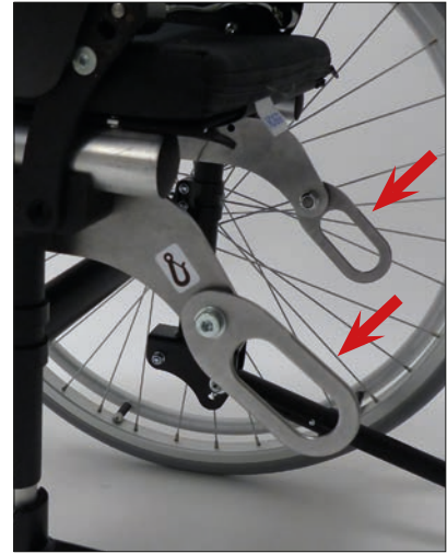
Attachment points, rear according to ISO 7176-19
