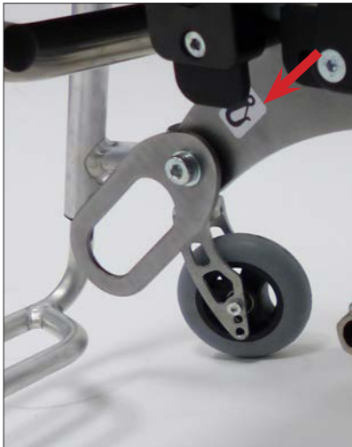
Attachment points, front according to ISO 7176-19
