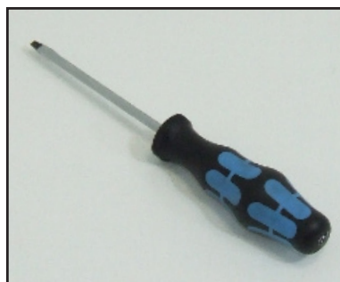
Screwdriver Blade width 2.5 3.5 and 5.5
