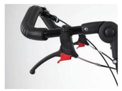
Each drum brake is operated by a brake lever.
