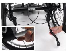
The anti tip supports are pre-assembled. Stick the anti tip tubes into the particular support. Press the snap button and choose the desired length position (please see close up picture).
