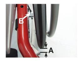
When the wheel lock is released the brake shoe should be 12-15 mm from the wheel (A).
