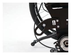
Picture shows the position of the anti tip. The anti tip should be adjusted that it is 2-3 cm above the ground.
