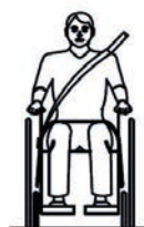
Illustration of proper belt restraint fit
