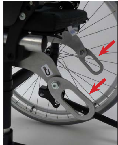
Attachment points, rear according to ISO 7176-19
