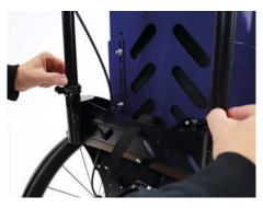
• Press in the spring button and slide the push bar / push-handle downwards fully into its bracket, until it clicks into position.
