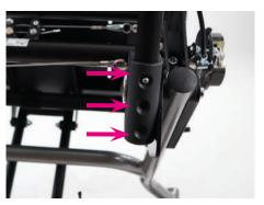
After pressing the snap button the length of the tubes can be adjusted in three positions (with respectively 2,5 cm distance).
