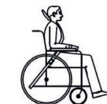
Illustration of proper belt restraint fit
