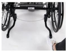
• Move the tubes with your foot to the top until the bolt clicks into the "passive" position.
