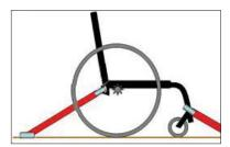
4) The buggy has to be fixed with a restraint system referred to ISO 10542 or SAE J2249 with fixed belts in the front and adjustable belts in the back.
