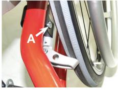
The brake shoe presses on the tires and grips it tightly. The brake shoe is, therefore, at a 90° angle to its holder. The brake shoe should overlap 3-5 mm to the middle of the wheel.
