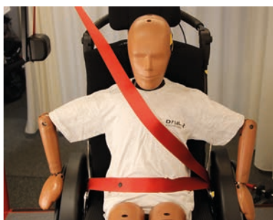
Occupant belt restraints must not be held away from the body by wheelchair components such as armrests or wheels
