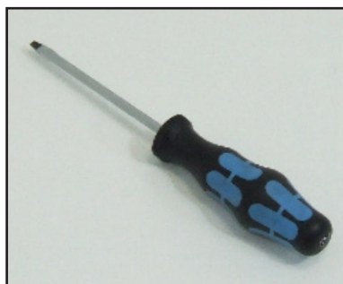
Screwdriver Blade width 2.5 3.5 and 5.5
