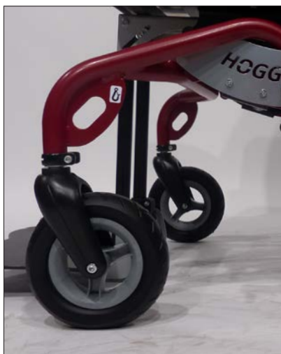
Attachment points, front according to ISO 7176-19
