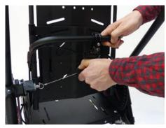
• Turn the toggle lever on the backrest and let engage the backrest in the first position.
