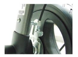
After loosening the counter nut the initial tension can be adjusted by screwing the guide of the bowden cable.
