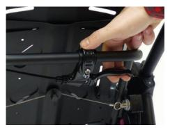
After pulling the active handle the angle of the seat unit can be adjusted.
