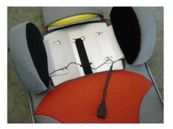
The stereo headphone can be retrofitted in headrest supports with spacer fabric.
