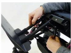
Activate the wheel lock of the BINGO Evolution Mini and position in front of the seat. Secure footrest and knee angle assembly with one hand before you loosen the toggle lever with the other hand. Swing the footrest to the desired position and tighten the toggle lever firmly again.
