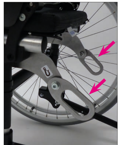
Attachment points, rear according to ISO 7176-19
