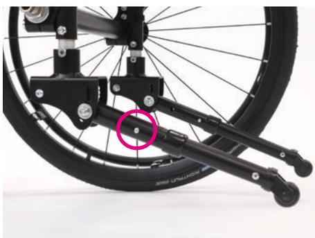
Press the snap button and choose the desired length position. The length of the anti-tipper tubes can be adjusted in the anti-tipper bracket in three positions 2.5 cm apart.
