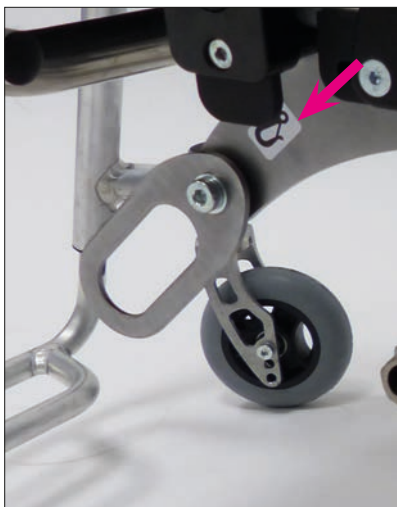
Attachment points, front according to ISO 7176-19
