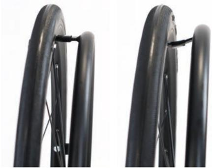
Push rims can be supplied with a standard diameter or with a larger diameter.
