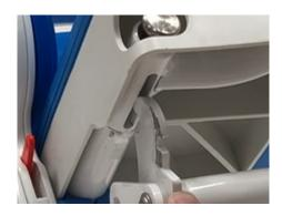
Make sure that the openings are hooked behind the locking shafts of the seat frame.
