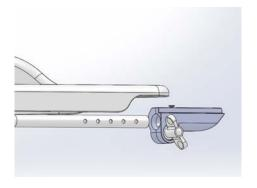
• Place the ventral upper body support with the frame construction in the holders below the armrest pads.
