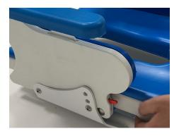
• Place the seat unit on the front locking shafts and finally let it snap into place.
