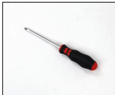
Screwdriver Blade width 2.5 3.5 and 5.5
