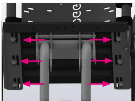
The wheelchair will be built in accordance with the customer's order. It is possible for the dealer to modify the camber of the rear wheels.
