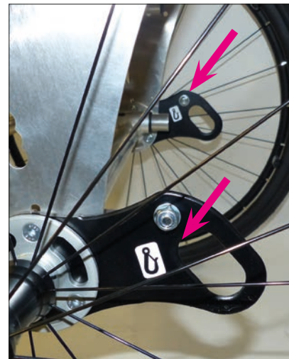
Attachment points, rear according to ISO 7176-19
