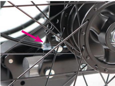
The brake force can be adjusted by the adjustment screw.
