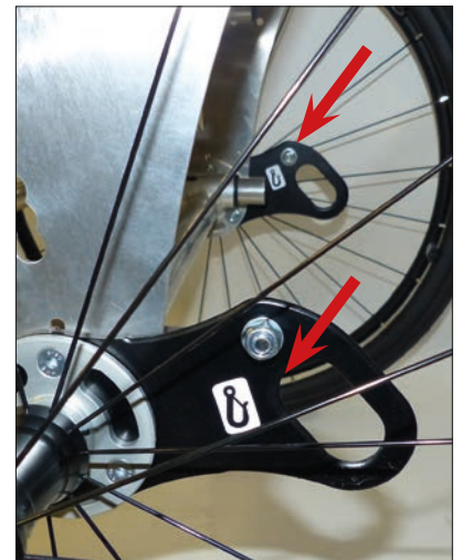
Attachment points, rear according to ISO 7176-19
