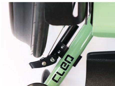
When the wheel lock is released the brake shoe should be 12-15 mm from the wheel.
