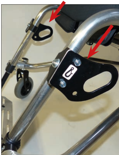
Attachment points, front according to ISO 7176-19
