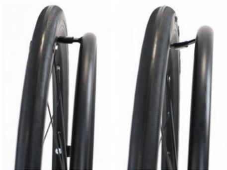
Push rims can be supplied with a standard diameter or with a larger diameter. These are called respectively hand rims “standard” or push rims “high”
