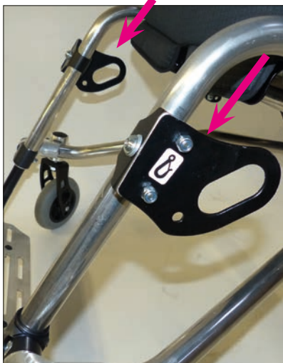
Attachment points, front according to ISO 7176-19
