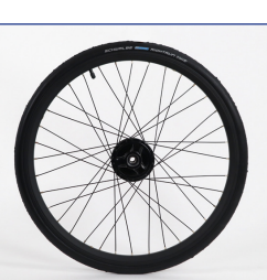
Flat free tires with drum brakes
