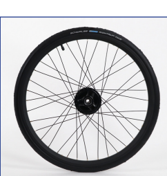
Pneumatic tires with drum brakes
