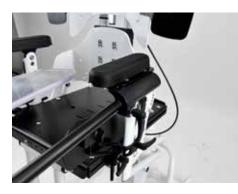
• Place the therapy tray with the frame construction in the bracket below the armrest pad.
