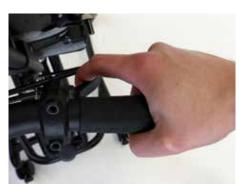
• Operate the right release lever as shown and move TIMO to the maximum seat height position.
