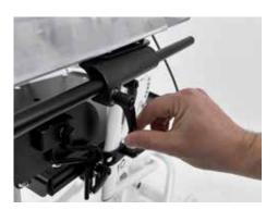
• Make sure that it is securely locked in place by tightening the clamping lever.
