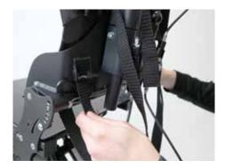
• Pass the lower straps under the backrest base from front to back and insert them into the open folding buckles above the locking bolt of the backrest angle adjustment.
