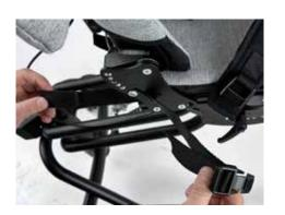
• Guide the tensioning strap from the outside with the side that does not have a loop through the slotted holes of the side plate of the back base on the right and left (see also 5.26 Lap belt).
