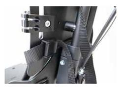
• The centre "axillary straps" must be threaded at the appropriate height between laterally along the attachment back plate.
