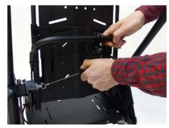
• Turn the toggle lever on the backrest and let engage the backrest in the first position.
