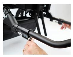
• Press the release buttons of the quick-release connections with your thumbs at the same time and allow them to snap into place.
