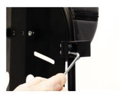
• Tighten the canopy adapters firmly. Proceed in the same way on the other side.
