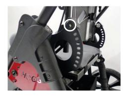
• The picture or the mark shows the backrest locked in the first back angle position.
