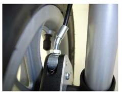
At the exit of each brake housing a cranked set screw leads the brake cable away from the tyre of the rear wheel. After loosening the counter nut the pre-tension of the individual (left or right) brake can be adjusted.
