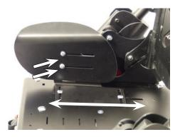
After loosening the wing nuts under the seat the hip supports can be adjusted concerning the depth continuously variable. After loosening the marked screws it is possible to adjust them also on the bracket.
