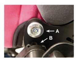
Attach the seat unit on the street frame and make sure, that the guide shaft (A) slides into the (tilt) bracket (B) on both sides.
