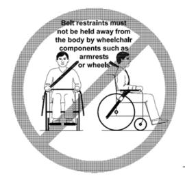
Belt restraints should make full contact with the shoulder, chest, and pelvis and pelvic belts should be positioned low on the pelvis near the thigh-abdominal junction.
