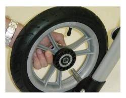
• To detach press the quick release spring towards the middle of the wheel and pull the wheel from the axle.
