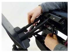
Activate the wheel lock of the BINGO SWITCH MINI and position in front of the seat. Secure footrest and knee angle assembly with one hand before you loosen the toggle lever with the other hand. Swing the footrest to the desired position and tighten the toggle lever firmly again.
