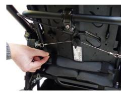
• Guide the Velcro fasteners through the long hole as shown and fix it.
