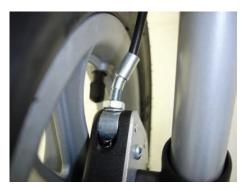
At the exit of each brake housing a cranked set screw leads the brake cable away from the tyre of the rear wheel. After loosening the counter nut the pre-tension of the individual (left or right) brake can be adjusted.
