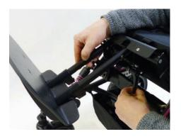
If your **BINGO SWITCH** is equipped with an angle adjustable footrest hanger the footrest could be in a hinged position for the transport.
