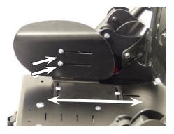
After loosening the wing nuts under the seat the hip supports can be adjusted concerning the depth continuously variable. After loosening the marked screws it is possible to adjust them also on the bracket.
