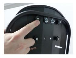
• Fix both coach bolts with the knurled nuts on the back of the backrest plate as shown.
