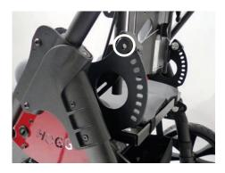
• The picture or the mark shows the backrest locked in the first back angle position.
