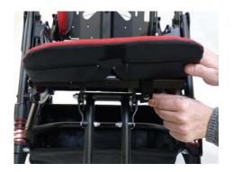
We recommend to adjust the seat unit in the desired position before attaching the upholstery. (Back tilt and seat tilt - see chapter 5).
