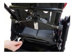
• Also attach the seat cushion with the snaps to the seat panel below the rear seat edge as shown.
