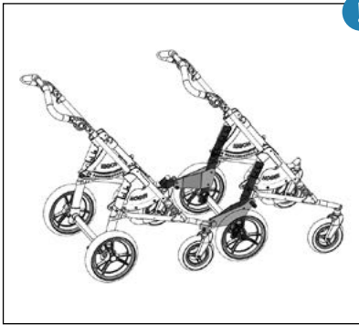
Connecting parts for 2 BINGO Evolution mobility bases incl. swivel lock on rear mobility base
