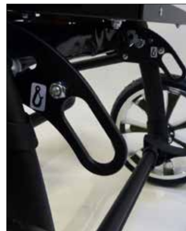
Attachment points, rear according to ISO 7176-19
